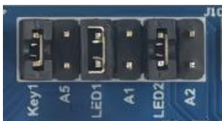
Figure 2 From Default LED1, LED2, KEY Resources to A1, A2, A5
