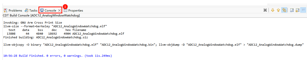
Figure 20 Successfully Compiled Example under Eclipse
